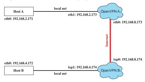
Host A (B) represents one of the machines that belongs to OpenVPN A (B). The two remote subnets are configured for a different range of IP addresses. When this setup is moved to a public network, the external interfaces of the OpenVPN machines should be configured for static IPs, or connect to another device (such as a firewall or DSL box) first.
