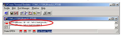
2. Type **#vi interfaces** to edit the network configuration file with vi editor. You can configure UC-7408's Ethernet ports for **static** or **dynamic** (DHCP) IP addresses.
