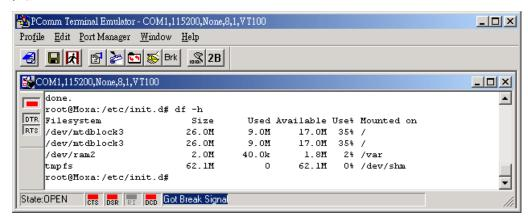
If there isn't enough "Available" space for your application, you will need to delete some existing files. To do this, connect your PC to the UC-7408 with the console cable, and then use the console utility to delete the files from UC-7408's flash memory.
